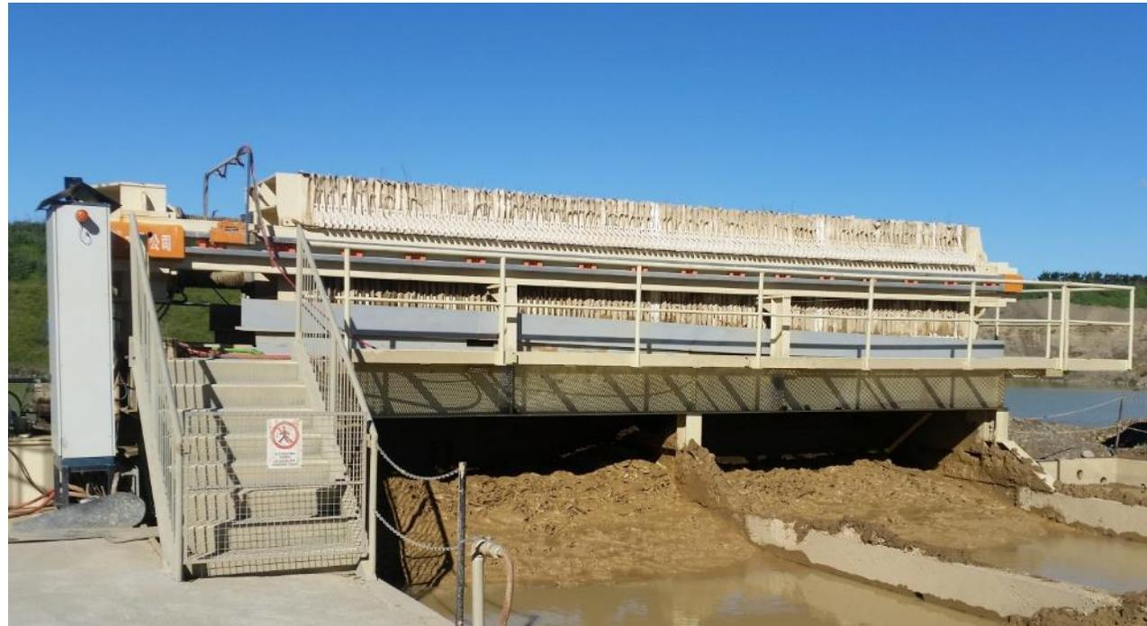
We introduced a water silo treatment system on one of our sites so we could reuse our water instead of it going to waste but found that this then filled our pond up with mud, so we continued to improve our site by introducing a filter press. The only waste we have now is around 10,000 lts of waste water a day compared to 950,000 before the press.
