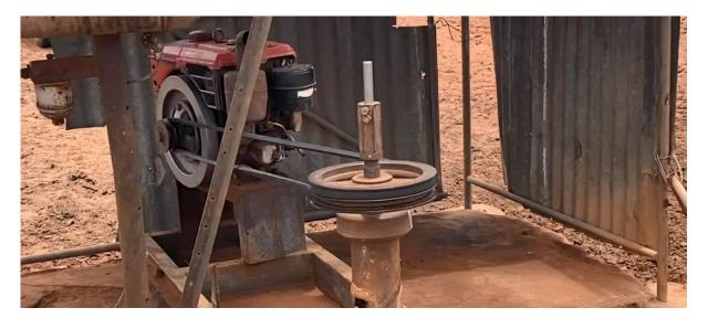
**Image 1:** The pump's moving pulleys and belt unguarded, are a hazard for nearby workers. (Source: NT Police)
