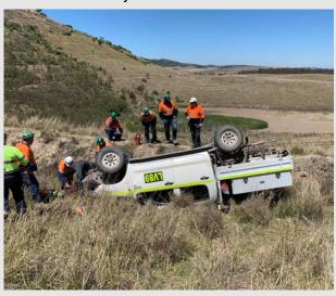
Vehicle operators must remain vigilant of the risk of rollovers and should be reminded of the importance of wearing seatbelts. When planning tasks and travel paths, supervisors must consider roll over hazards.
