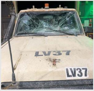
The risk of collision when vision is restricted is well documented and reasonably foreseeable. Suitable risk controls such as cameras and vehicle escorts should be used when tramming large items of plant with restricted visibility around mine sites.
