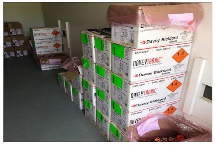
The use and storage of explosives is regulated under the Health and Safety at Work (Hazardous Substances) Regulations 2017- 9.27. We also recommend that storage of explosives should also be carried out in accordance with AS 2187.1-1998 Explosives - Storage, Transport and Use. This standard covers the requirements for magazines, segregation and separation distances, and emergencies.
