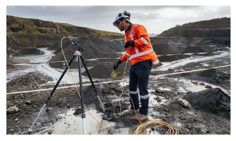
All blastholes must be measured prior to charging, in the event that re-drills or adjusted charging is required. If measurement was carried out prior to the day of charging, and a physical change to the blasthole is likely (e.g., following a rain event), then it is recommended that blastholes be re-measured prior to charging.
